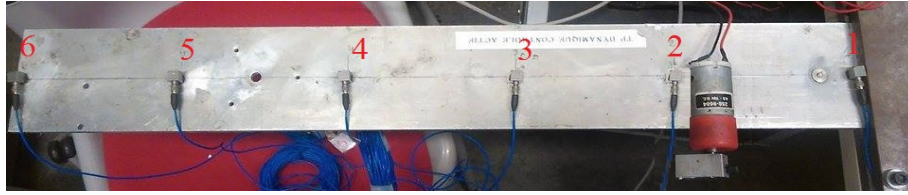
Figure 1: Experimental setup for the cantilever beam structure
