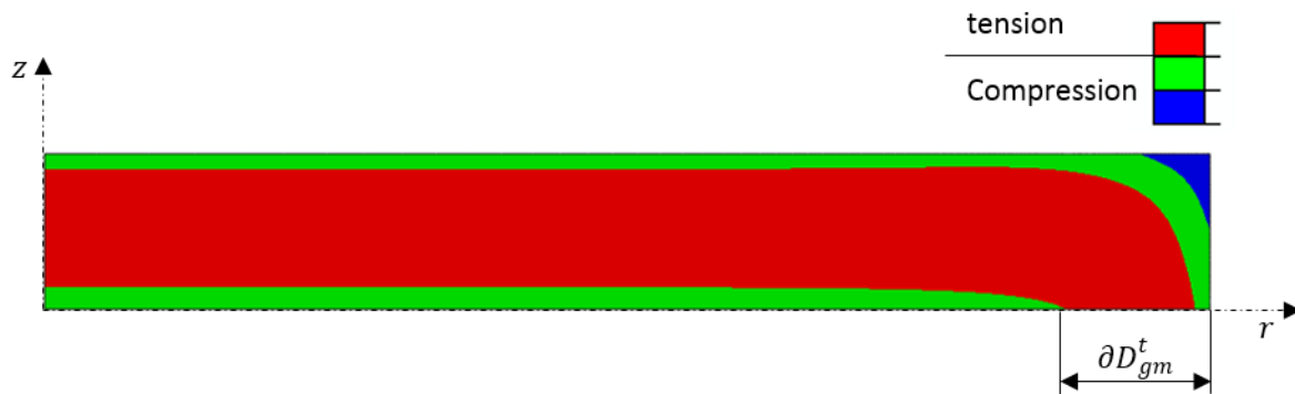
Figure 8: Circumferential residual stress distribution in the glass supported by the mold ring of R_1 = 40 \text{ mm}
