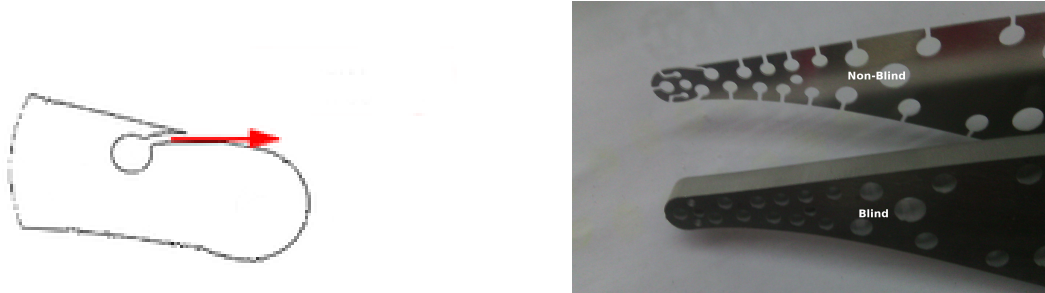
FIGURE 2 – Left : diagram of a thin (non-blind) profile. Right : photograph of the thick (blind) and thin (non-blind) profiles.
