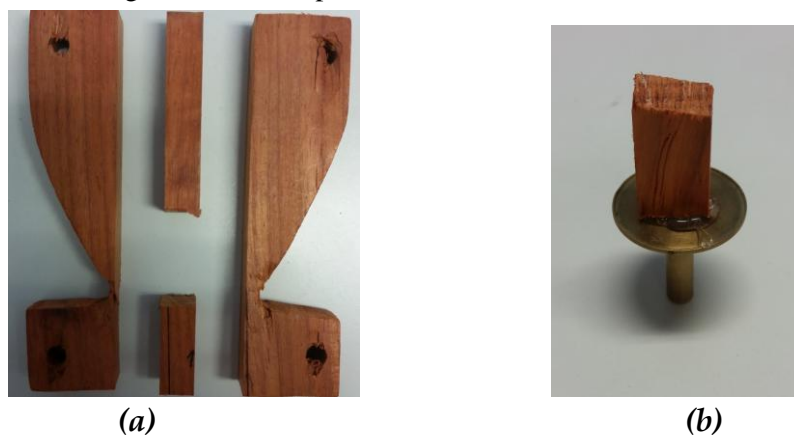
Fig.2: 3D image acquisition protocol by X-ray microtomography (from right to left): Cutting of the specimen and location of the sample, sample of wood to be scanned by XCT.
