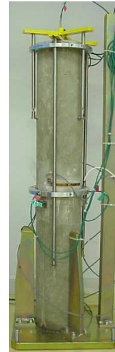
Figure 2: Drying shrinkage test
