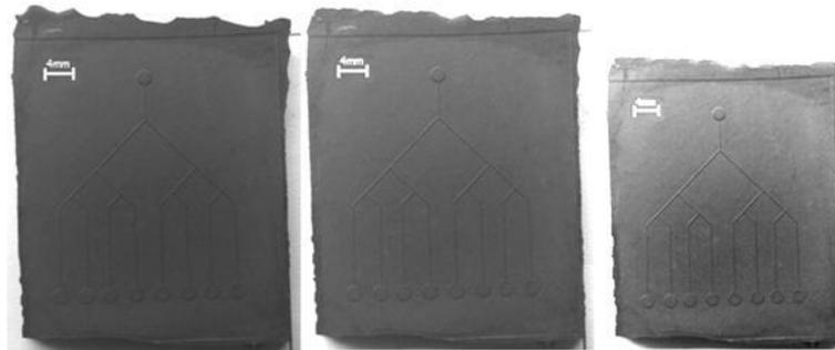
Fig. 8. Photographs of the micro-fluidic replicas after the: (a) embossing (b) debinding and (c) sintering steps, which were produced using 316L stainless steel feedstock (solid loading : 64%).
