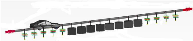
Fig. 4 Numerical model for crashing test of the VRS
