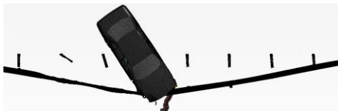
Fig. 8 Failure of vehicle redirection when H and E decrease
