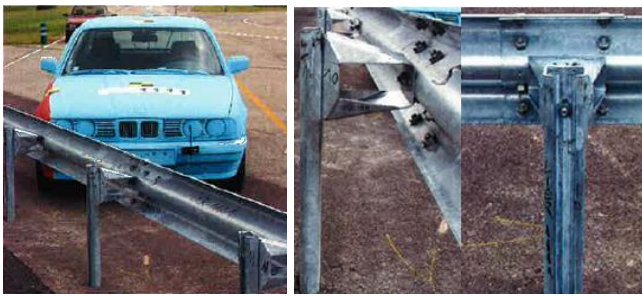
Fig. 3 The VRS evaluated by crash test with vehicle
