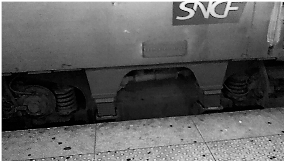
Figure 1: Stack-layered rubber-steel 2 ary suspension blocks on SNCF's BB 22000 series [own work].
