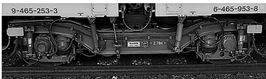
Figure 2: Concentric-layered rubber-metal 1 ary springs on Renfe's CIVIA series [7]
