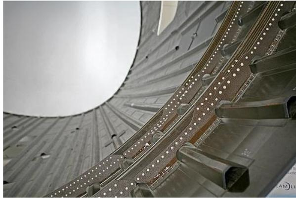
Figure 1: Application of hat stiffened panel in fuselage Boeing 787
